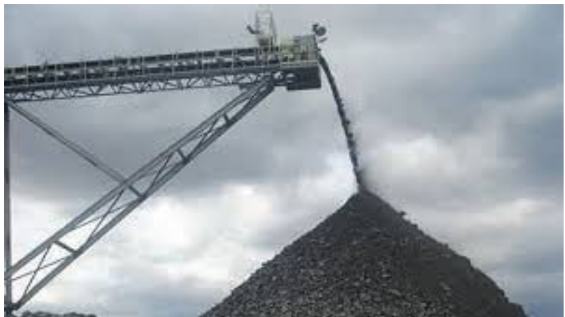
Figure 1: Cone formation (Image from masoncontractors.org )
